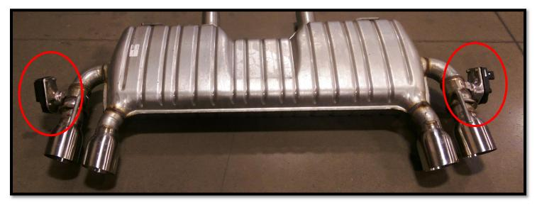
**STEP 3.** Factory Muffler removal
